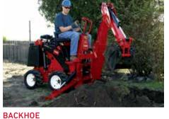
Versatile — dig foundations, plant trees, trench and much more. Folds to 34.5" wide for access to tight spaces and ease of transport. 180° bucket and swing arm rotation, 82" digging depth and standard 13" bucket. Stabilizer spread: 78"
