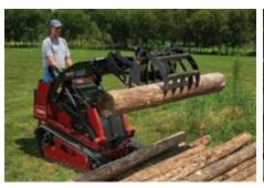
**GRAPPLE RAKE** Grab, drag, lift and place brush and debris easily with up to 3,000\* lbs (1,361 kg) of clamping force at the tine tips.
