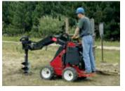
**IMPROVED VISIBILITY** platform allows improved visibility of the working area and attachments.
