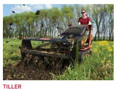
Hardened steel tines for any soil condition, including clay or hardpan. Till more than 6" deep and 40" wide on one pass. Reversible tine direction frees jams quickly. Tine speed: 175 rpm @ 8.5 gpm
