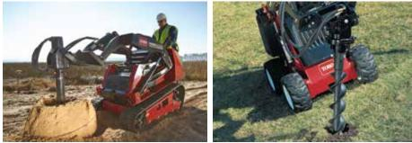
Auger bits from 6" to 30". Bit speed: 54 rpm @ 11 gpm
